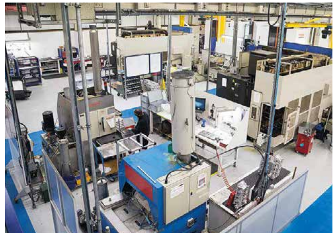
Low volume automotive production cell: major casting machining – GE Precision Engineering
