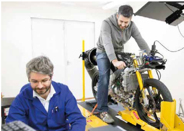
Moto3 engine testing on GE Precision Engineering's motorcycle chassis dynamometer
