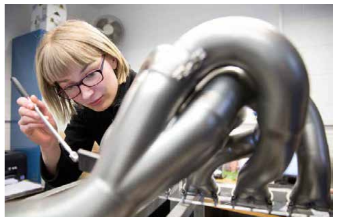
Inspection of shot peening on a racing exhaust system – Sandwell
